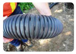
Weeping tile is a perforated plastic pipe or clay tile pipe that runs underground along the bottom of a home's footing. As water percolates down through the soil, the water flows into the holes/gaps in the weeping tile and is drained away from the foundation of your home. Weeping tile is typically connected to a sump pump and a sump pit and drains either into the storm sewer or into a dry well. It is important to disconnect any weeping tile that may be connected to the sanitary sewer main.
