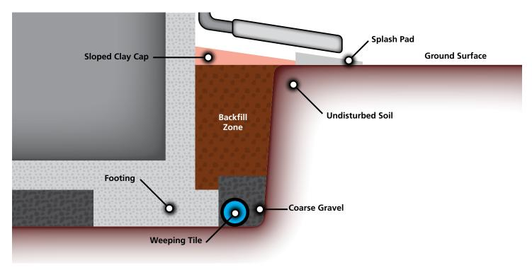
of silt and clay. This problem is more common in areas with silty and clayey soil. The most common problems with weeping tile drainage are associated with the sump pump and sump pit rather than with the weeping tile
